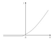
Axes labelled, very low current for negative voltages / increasing current for positive voltages
