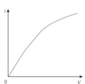
Axes labelled, straight line curving at high current with decreasing gradient
