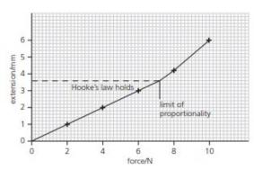
c Gradient calculated by triangle method using at least half of linear portion of graph [1]; gradient = rise/run =  $2 \times 10^3$  N/m [1]
