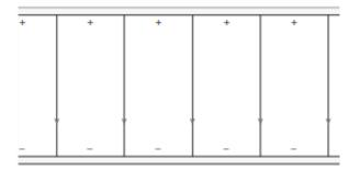
Parallel plates with opposite charges perpendicular field lines, direction of field marked correctly
