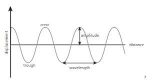
Crest, trough, amplitude, and wavelength correctly labelled
