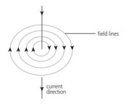
Circular field lines around wire, field direction and current direction marked correctly
