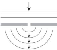
Curved waves [1] extending into region behind barrier [1] with same spacing as incident waves [1]
