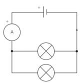
Correct symbols used for: battery, ammeter and two lamps lamps connected in parallel, current direction marked correctly with arrow
