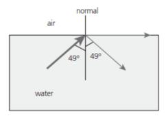
Normal, incident and reflected rays drawn correctly at boundary critical angle (49°) marked
