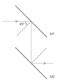
Reflected ray at M1 [1] normal at M2 [1] and reflected ray at M2 [1] drawn with incident and exit rays parallel [1]
