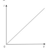
Axes labelled, straight line with positive gradient through origin
