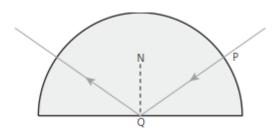
Ray reflected from Q [1] and exiting glass normally [1] correctly drawn
