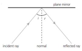
The plane mirror, the incident ray, the normal to the mirror, the reflected ray, the angle of incidence, i, and the angle of reflection, r, correctly labelled
