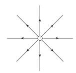
Positive point charge radiating field lines, direction of field marked correctly
