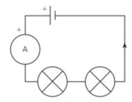
Correct symbols used for: battery, ammeter and two lamps lamps connected in series, current direction marked correctly with arrow b
