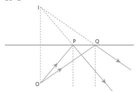
Normals to mirror at P and Q, reflected rays at P and Q, extrapolated rays at P and Q correctly drawn, image position correctly located
