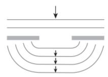
Straight waves passing through gap [1] curving into region behind barrier [1] same spacing as incident waves [1]
