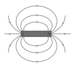
Field lines correctly shaped, N and S poles marked, arrows showing direction of field correctly
