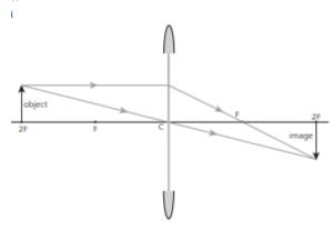
Principal foci (F) and optical centre (C) marked [1] construction rays [1] object [1] and image [1] correctly drawn
