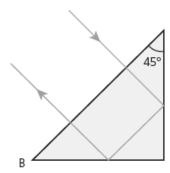
Prism A: reflection of ray at sloping surface [1] transmission of ray at exit [1] correctly drawn
