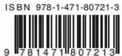
Figure 6.14 Barcodes are made up of alternating dark and light lines of varying thickness
