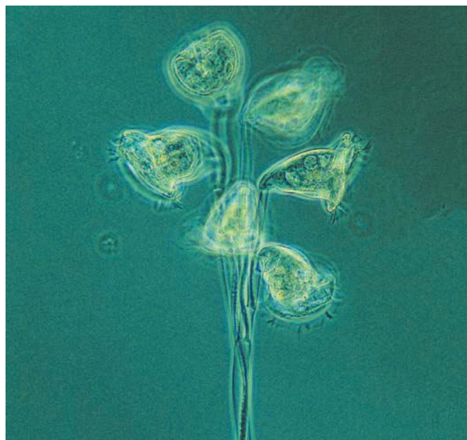
Figure 21.37 Protocista in activated sludge ( \times 150 ). These single-celled organisms ingest bacteria in the liquid sewage.
