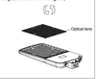
Step 3.Put back the adjusted optical lens, lock screws back, as shown in the figure.
