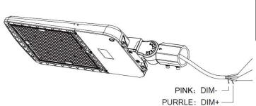
As for the wire color of DIM + and DIM - , pls check the lamp label!
