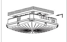
5. Secure the screw. Installation complete
