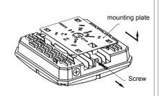
2. Use screws to lock the mounting pla on the embedded junction box.
