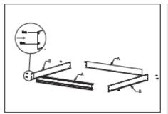
① Assemble the surface mounted frame and fix by screws.
