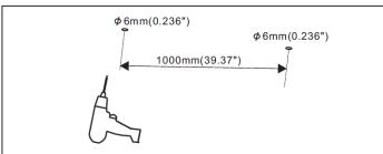
1.Drill the hole on the ceiling (The size is shown in the picture)
