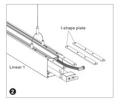
Insert the I-shape plate to the track as the picture shows.
