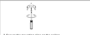
3. Secure the mounting clips on the ceiling
