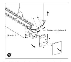
Install the Linear 1 to the ceiling as instruction of Suspension Installation. Open the end cap as the picture shows. Pull out  $\frac{1}{2}$  Power supply board of Linearl, and move out the AC wires. Disconnect the A and B parts.
