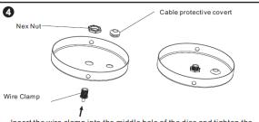
Insert the wire clamp into the middle hole of the disc and tighten the wire clamp with hex nut; Clip the cable protective cover into the AC line hole of the disc.
