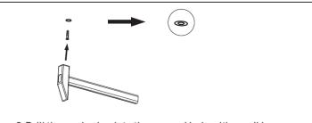
2. Drill the anchoring into the opened hole with a nail hammer
