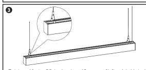
Rotate and fasten 2 fixing heads and 2 screws of left end; hold steel wire rope and lift lamp upward, then adjust balance screws to balance light, finally tighten balance screws.
