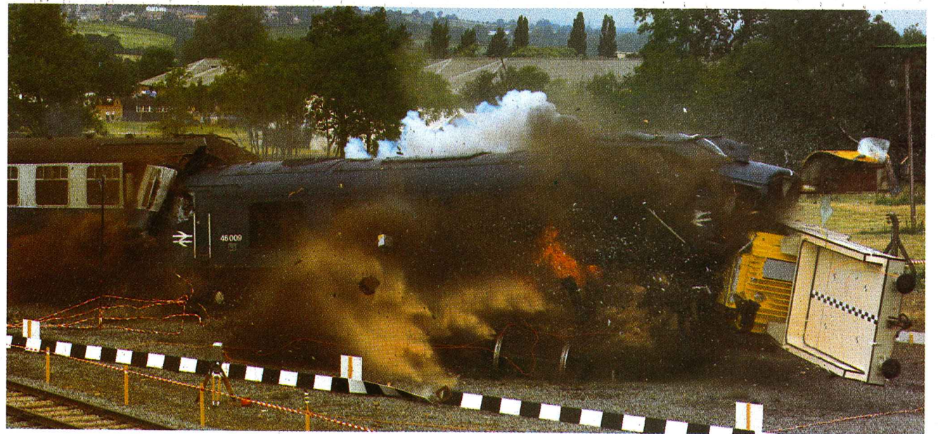
A spectacular demonstration of the safety of transporting spent nuclear fuel by rail from nuclear power stations for reprocessing was held in 1984. Watched by millions on television, a heavy diesel locomotive pulling three passenger carriages was driven at 100 miles an hour into a nuclear fuel flask as it lay on the test track at Old Dalby in Leicestershire. The loco was crushed but the flask remained intact.
