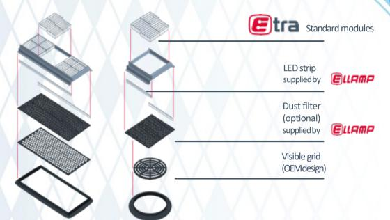
Fully custom modules made according to client reequipments. (used were standard ETRA modules are not applicable
