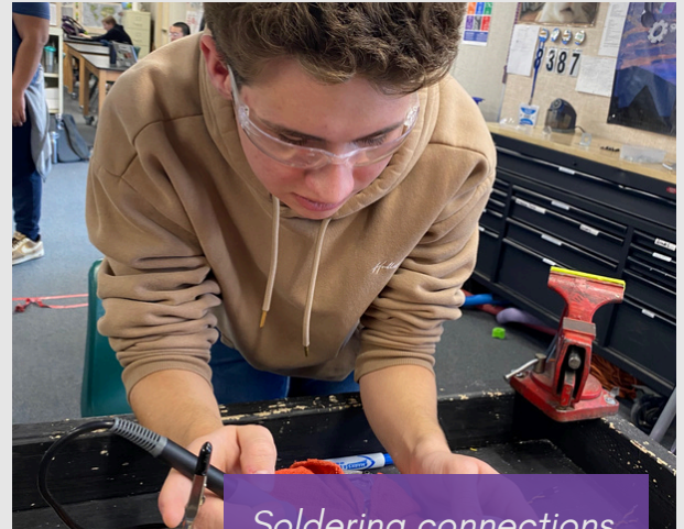
Soldering connections on the robot
