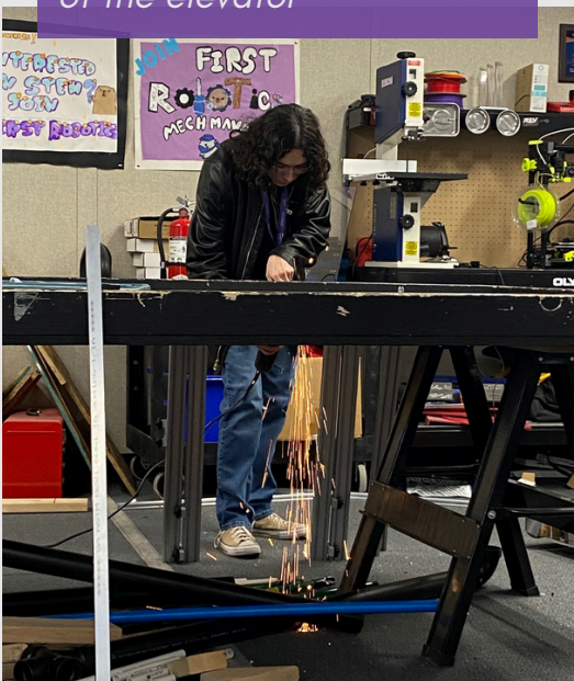
Grinding down parts of the elevator
