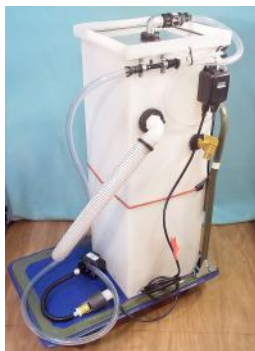
6. Portable Coalescer for Tramp Oil Removal and Filtration of a 24-7 Production CNC
