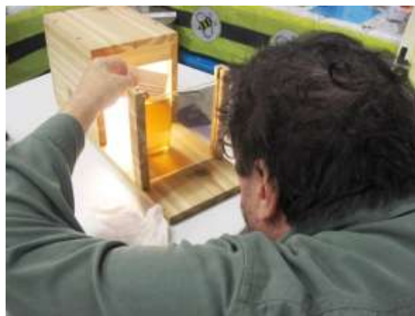
Above left, crystals seen through a polariscope (Image: Wyatt E. Mangum, 200 Top Bar Hives: The Low-Cost Sustainable Way); right, Peter uses the club polariscope built by Martin Stenzig to assess crystallization in an entry.
