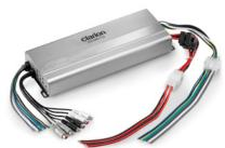
5-Channel, Class D System Amplifier Main Channels: 50W x 4 @ 4 ohms / 75W x 4 @ 2 ohms Subwoofer Channel: 200W @ 4 ohms / 300W @ 2 ohms
