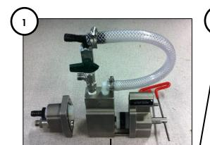
Disassemble the Power Survivor according to chapter "Seal Replacement" in the manual.
