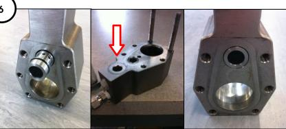
Push the valve sleeve by hand into the pump housing until it goes stiff. Turn the assembly on a flat ground and push down until the spool valve is flush to the pump housing.
