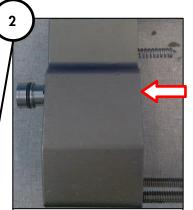
Push the valve sleeve out of the housing. It's very stiff!
