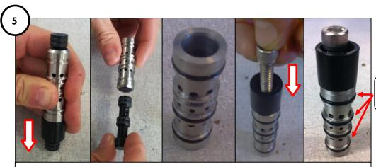
Remove the old spool valve from the sleeve.
