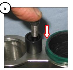
Use the screw as an extension to press the spool valve completely into the borehole.
