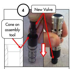
Place the valve sleeve with the cone end to a table and push the spool valve threw the assembly tool into the sleeve.
