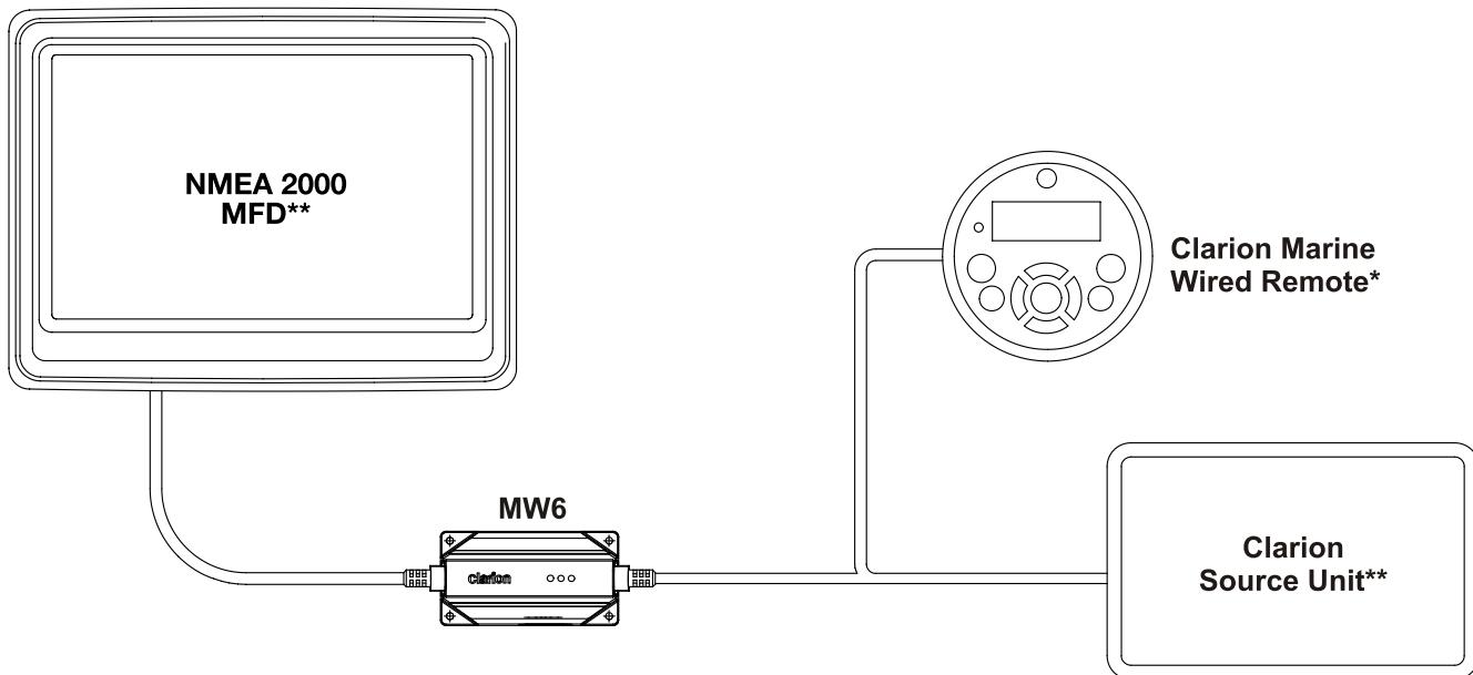
\* **Wired Remote can be connected via MWRYCRET "Y" Cable.**
