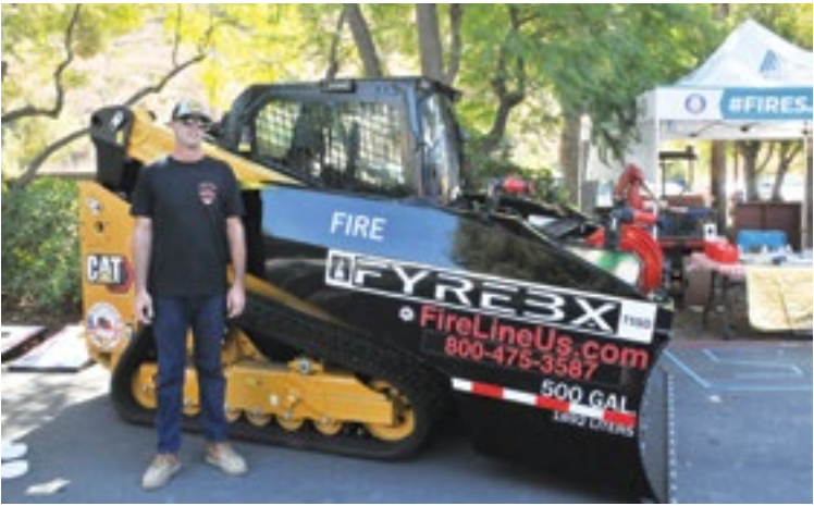
Chris Larocque of FireLineUs, explains the workings of the FyreBX, a compact fire-fighting track loader that holds 500 gallons of water, a hose reel, dozer blade, and equipment. It can assist fire agencies and property owners in clearing areas ahead of time or battling a blaze when it occurs.
