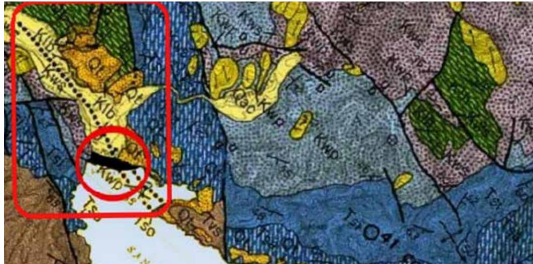
An earthquake fault, discovered in 1973, runs directly beneath the earthen Santiago Dam.
