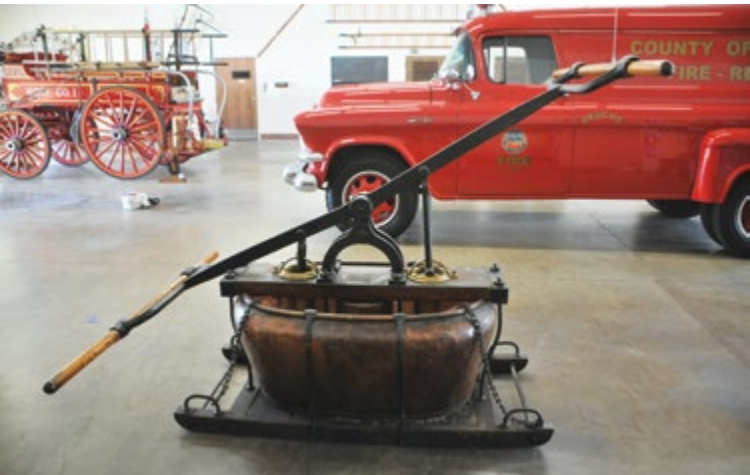
An 1850 French hand pump was fashioned on skids because the ground was either muddy or snowy, and wheels wouldn't work. The pump could throw water 30 to 50 feet through a riveted leather fire hose.
