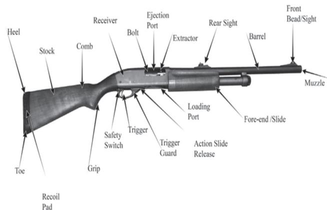
(Figure 2-5) Shotgun pump action nomenclature
