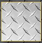
Diamond plate, also known as checker plate and is corrosion-resistant, anti-slip, hot-rolled, and suitable for a multitude of applications.
