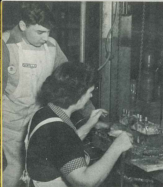
Thomas McLean, presently assigned to Dept. 32, is learning brazing as a part of his apprenticeship training. Photo pictures Gertrude Gesell showing Tom proper method for performing silver soldering operation.
