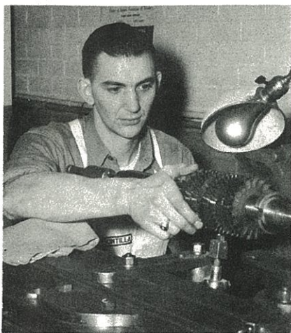
As an initial introduction to apprenticeship, George Muir learns cutter sharpening by acquainting himself with a cutter grinder in the Tool Room. Later he will actually operate grinder.
