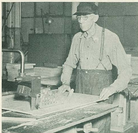
Guy Fitch, left, and Charles Brush try out the new Flohr Saw Guards recently installed in the Carpenter Shop. These guards automatically cling closely to the work, offering maximum protection. They are also equipped with a device which prevents kick-back. This equipment is approved by the New York State Department of Labor.
