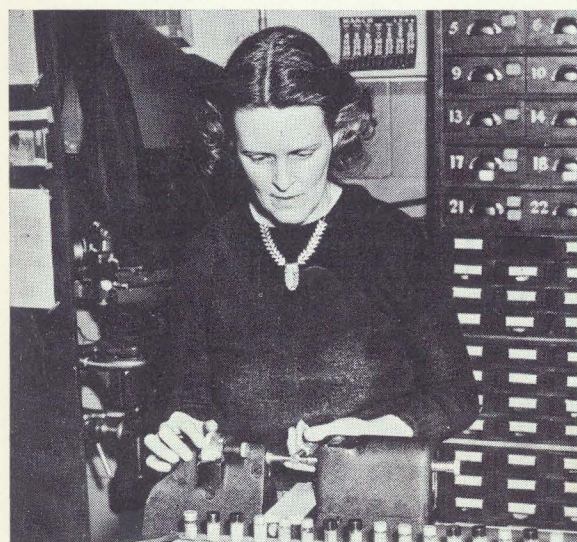
Inspecting Plug Gage on a "Supermike" in Gage Inspection Dept. Dorothy Morris is the Inspector.
