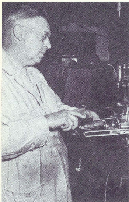
Following final assembly, William Lord subjects K-magneto to electrical test.
