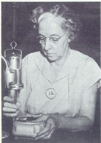
Ruth Brisack is pictured here as she places a cover on completely assembled K-magneto.
