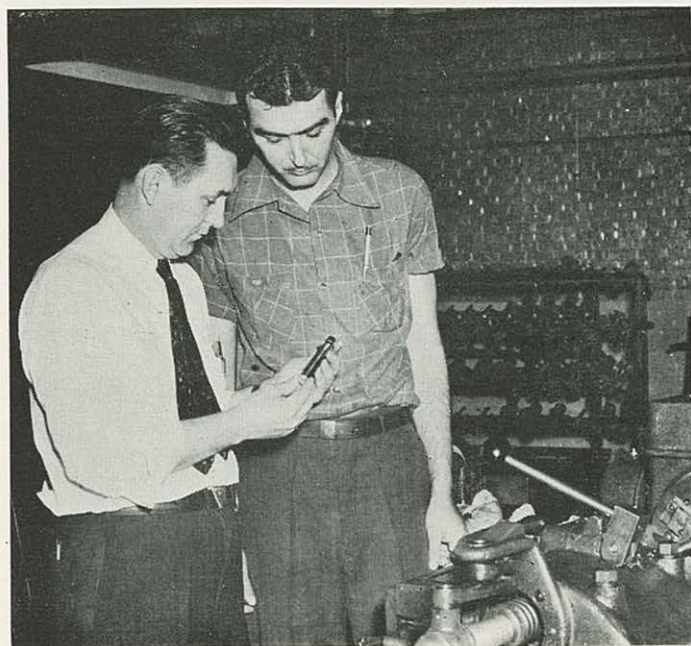
Walter Donnelly (left), formerly associated with the South Bend and Philadelphia Divisions of Bendix, examines a Fuel Injection Plunger Blank turned by Bob Ward (right) on a lathe. Carbide cutting tool was used for the operation.
