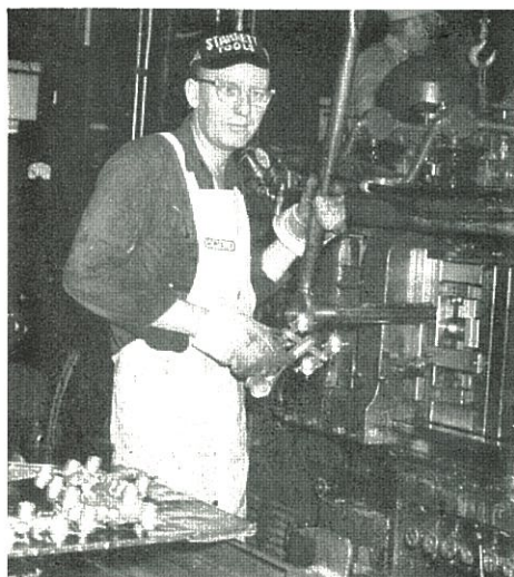
RALPH W. HANSON unloads gate of connector shells from Die Casting Machine in Dept. 37, has worked at plant since Sept., 1950.
