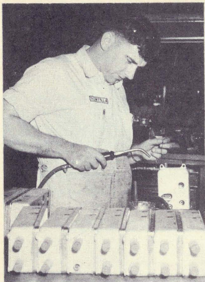
Bob Meehan of Dept. 42, performing a soldering operation, seals jet units airtight so that high altitudes will not affect operation of system.
