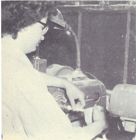
Other Ceramics operations on igniter plugs include baking, machining, burning and glazing. Leona Ellis, above, rounds off tip end of plug prior to burning.
