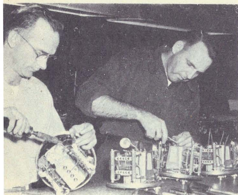
Paul Rodgers and Gordon Bronson, both of Assembly, are pictured assembling Exciter Units for another type of jet ignition system.
