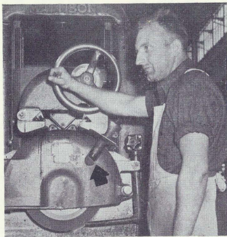
Above—Arrow points to diamond used in dressing grinding wheel. Rufus Baker, Tool Room, is pictured.
