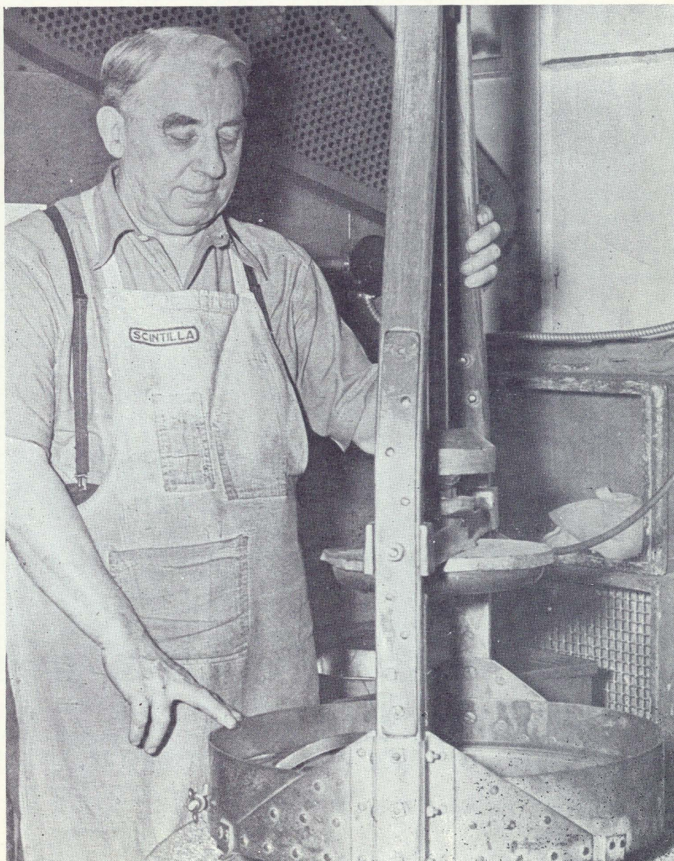
Above—A Consolidated Gear Press used for blanking flyweights from stainless steel. A pressure of 75 tons is exerted by the press in cutting each blank in this operation. Charles Ricks (21-4) is the operator. Inset— H. L. Scofield , 2nd Shift Foreman. Below—A veteran Scintillite, Walter Male (21-12) operates a "riddle" . . . a device used to remove shavings, chips, dirt, etc. from small parts. Mr. Male has been a Scintilla employee for about 16 years.
