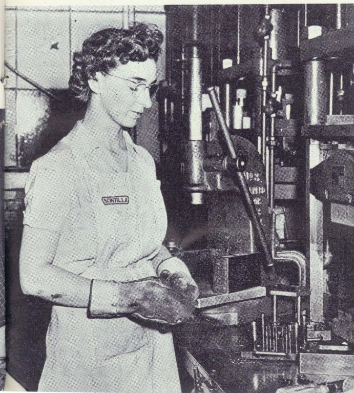
Above—Paul Miner, Department 24, transfer molding an Allison Distributor Finger with induction heated Melmac. Below—Isabel Finch, Department 24, molding small Insulator parts on a Compression Press.
