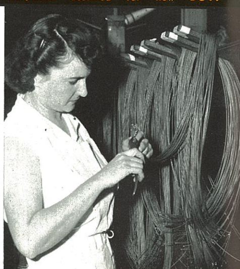
ANN HUGHES prepares wire sets in harnesses destined for new DC-7.
