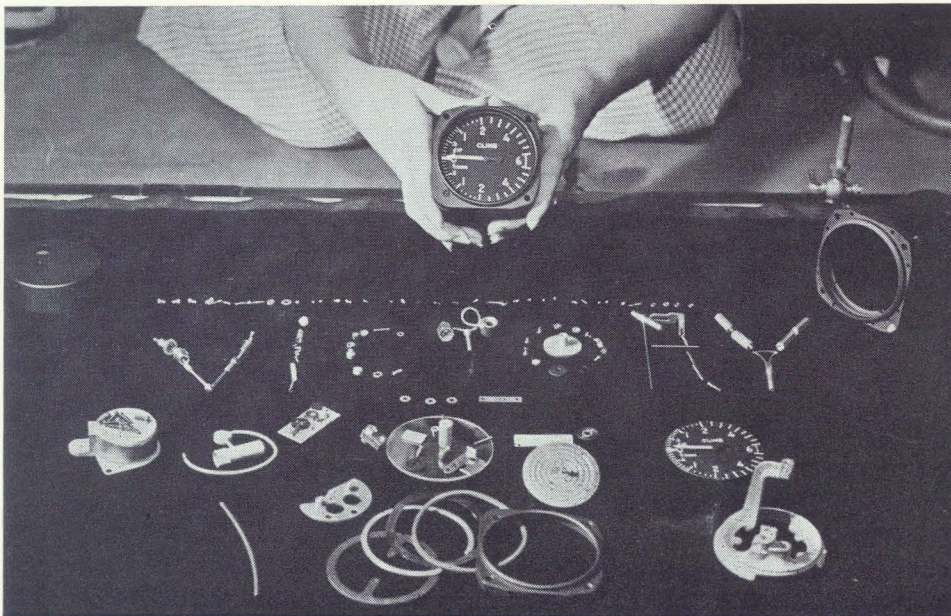
A Day's Work Under the Finger Nails . . . Many precision aircraft instrument parts are so tiny that, literally a craftsman can hold an entire day's work under his fingernails. Shown here are more than 140 parts that go into a Rate of Climb Indicator at the Philadelphia Division of Bendix Aviation Corporation, world's largest aircraft instrument plant. Put together, they spell a word that's on everybody's tongue. Look closely and you'll see it in the picture.
