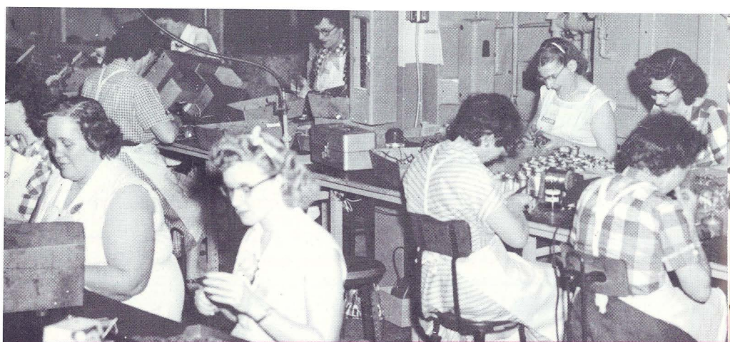
ABOVE GROUP is shown working on preliminary assembly of coils prior to filling with compound. Scene is typical of many operations in new Electronics Building.
