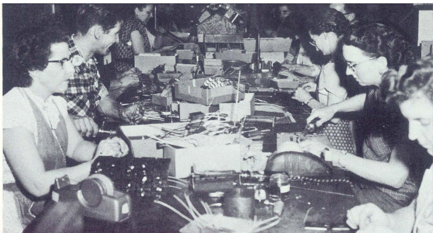
DEPT. 38 GROUP is pictured here making sub-assemblies for jet ignition units.
