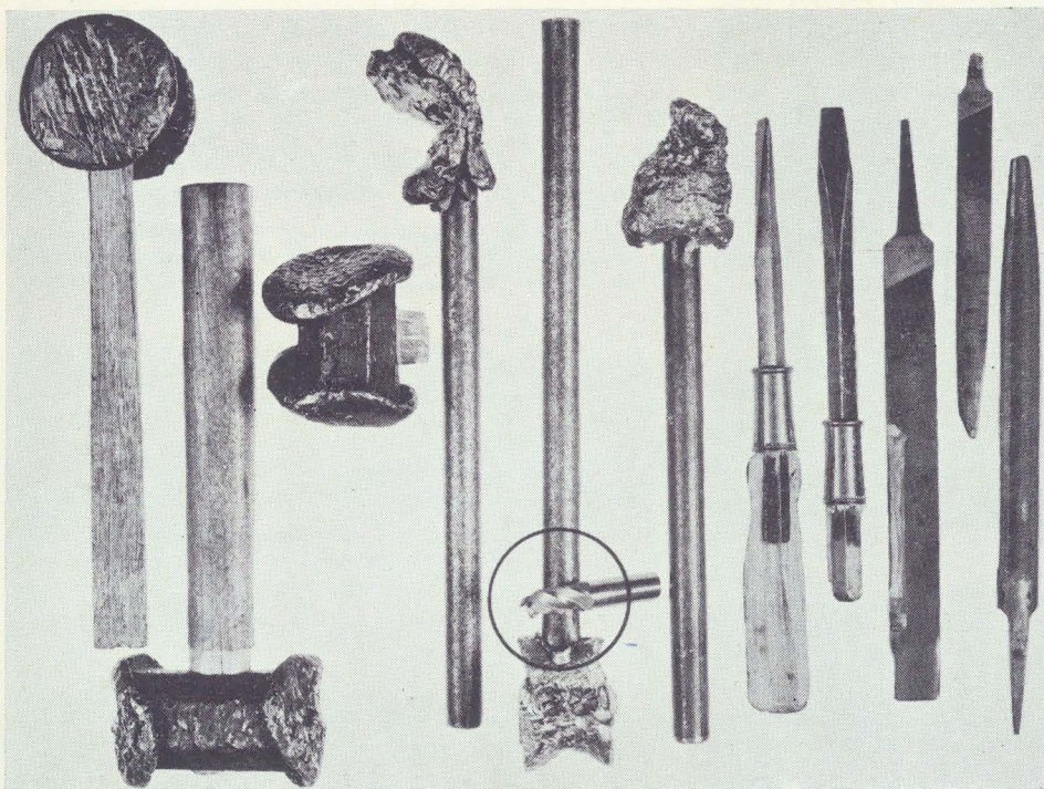
Examples of hazardous tools . . . accident breeders! Lead and brass hammers battered almost beyond recognition . . . screw driver handles split by prying . . . loose-fitting hammer handles. Proper care and use of tools is a MUST in the prevention of accidents.
