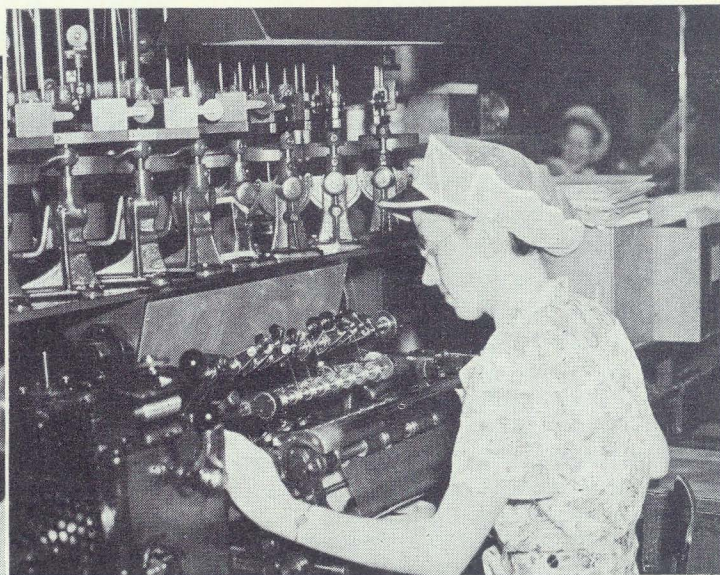
SLIGHTLY MORE COMPLICATED is this machine known as a multiple Coil Winder. The operator is Mrs. Evelyn Mitchell (15-170).
