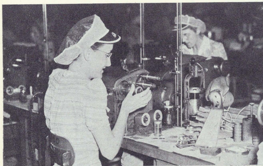
SECONDARY COIL WINDING is the operation in this photo. Mrs. Helen Bookhout (15-289) is the operator. This Coil requires about one mile of copper wire smaller than a hair in diameter.
