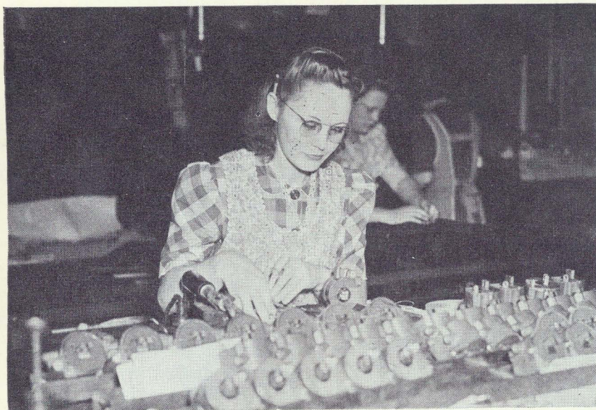
A JOB THAT REQUIRES meticulous care . . . soldering operation in Coil Assembly. Even a minor flaw in soldering can mean death to a flier if soldered part or wire gives way. Mrs. Vera Carr (15-471) is shown in photo.
