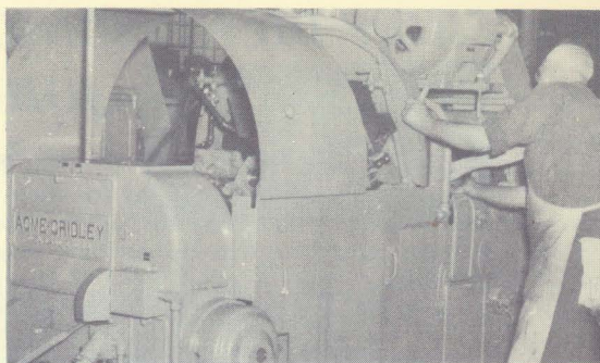
More and more, as we tour the Scintilla Scene, we find new machines and equipment everywhere throughout the plant. In Dept. 26 we took this photo of Joe Cooper and Jesse Decker making some adjustments on one of two new Acme Gridley Automatics received in that department. Both machines are single spindle bar type.
