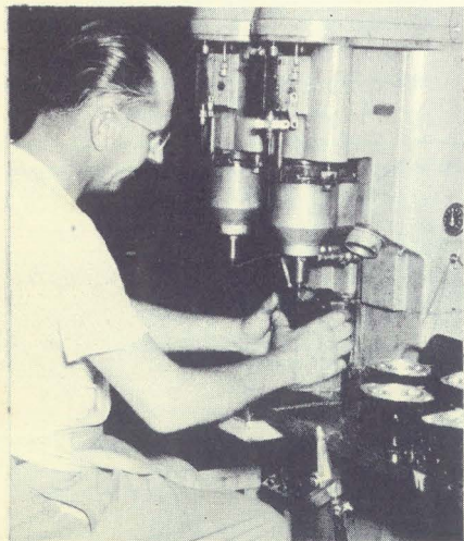
TAPPING OPERATION by Doug Drumm makes pipe thread holes in housing.
