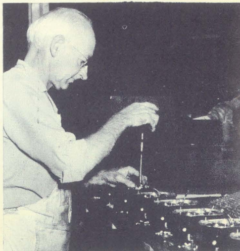
EDISON SMITH is pictured as he assembles breakers in tank magnetos.
