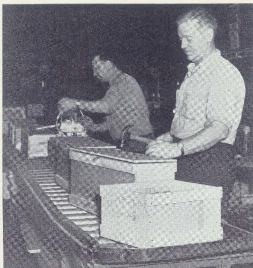
Wooden boxes pass down the packaging line for nailing. Otis Norton is pictured nailing covers in place.
