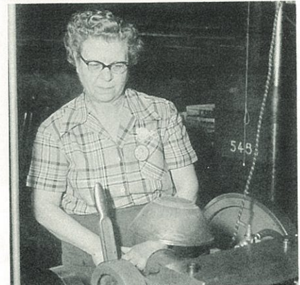
CASTLES from machine operated by E. Storrer in making connector clips.
