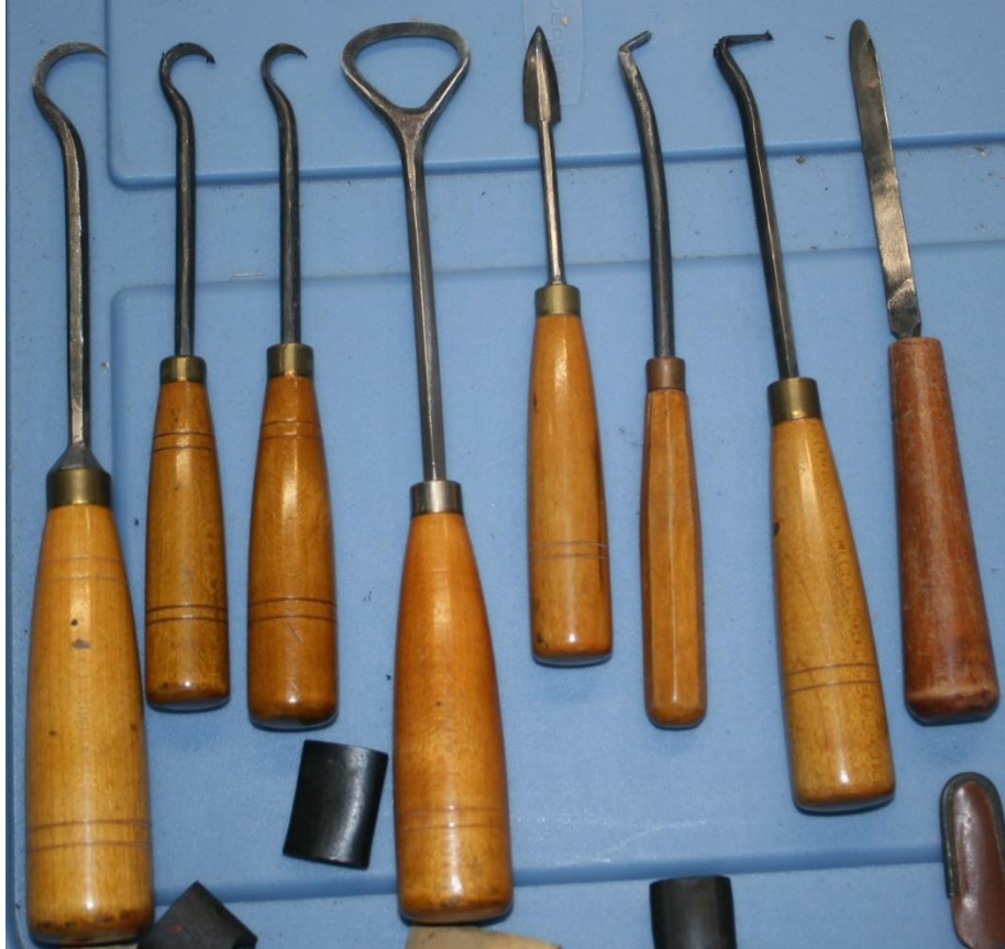
(left to right): 9" 2-Sided Scoop, 6 1/2" & 7" 2-Sided Scoops, 9" 2-Sided Loop Scoop, 6 1/2" 2-Sided Hook Knife, 8" Modified right & left side "L", 7" Side Chisel, Homemade Bullet-Point 7" Chisel
