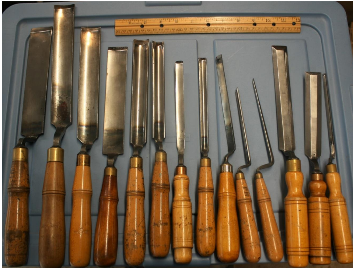
Large Gauges (some JB Addison) (left to right): 15"x1 1/2" Flat, 16 1/2"x1 3/8", 15"x1 1/4", 13 1/2"x1 1/4", 13 3/4"x1", 13 1/4"x3/4", 12"x1/2", 12 1/2"x 1/2", 12"x 1/2", 10 1/4"x1/4", 11"x3/16" Buck Brothers Flat Chisels: 13 1/2"x1", 11 1/2"x1", 11 1/2"x1/4"
