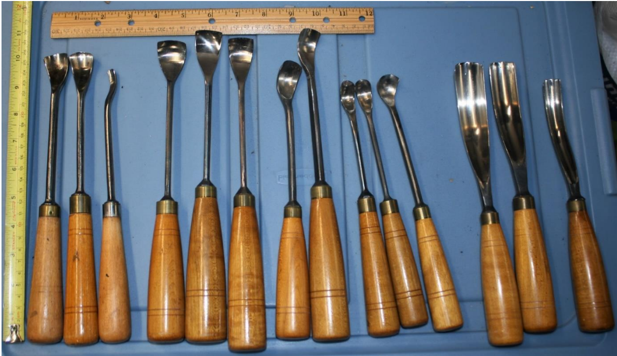
(left to right): JB Addison & Sons Tools: #9 10"x1" Scoop, #10 10"x7/8" Scoop DR Barton Tool: #28 9 1/2"x3/8" Scoop Unlabeled Carving Scoops 10 1/2"x1", 11"x1", 11"x7/8", 9 1/2"x3/4" Deep Scoop, 11"x7/8", 9 1/2"x1/2" Deep Scoop, 9"x9/16" Deep Scoop, 9 1/4"x7/8" Deep Scoop Large Sweep Gauges (left to right): 10"x1", 9 3/4"x7/8", 9"x5/8"
