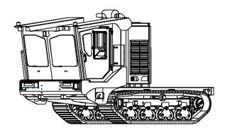
The Roughneck LP6 strong, multi-purpose, low ground pressure tracked vehicle operates efficiently in off-road and all-weather conditions.
