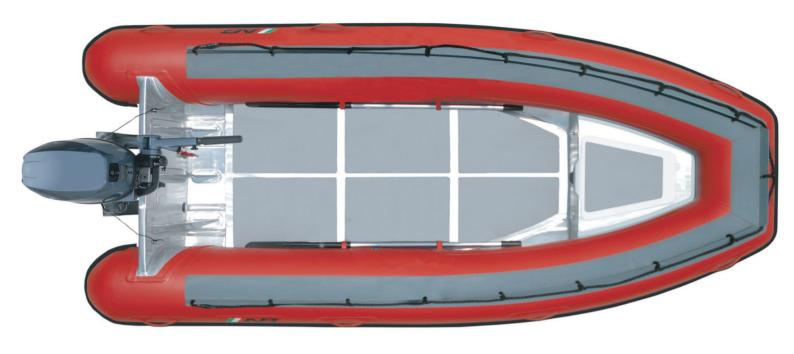
Overal Length Number of Chambers : 13'/ 3.96m Shaft Length : 20" / 50.8cm **Overal Beam** : 6'5"/ 1.96m **Person Capacity** : 7 RDC Design Category : C Inside Length : 9'10"/3.00m Weight : 282lb/128kg Inside Beam : 3'3"/ 0.99m Recommended HP : 30hp /22.4kw Maximum HP **Tube Diameter** : 18"/ 0.46m : 40hp / 29.8kw
