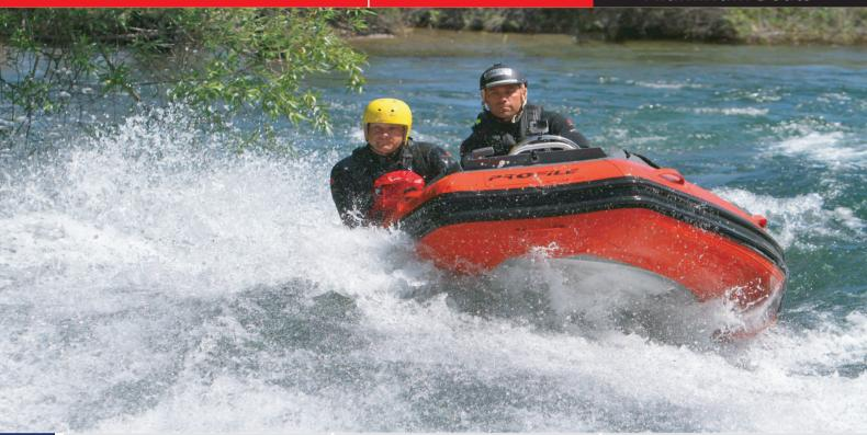
Overal Length : 14'/ 4.27m **Number of Chambers** Shaft Length : 20" / 50.8cm **Overal Beam** : 6'5"/ 1.96m **Person Capacity** : 8 RDC Design Category : C
