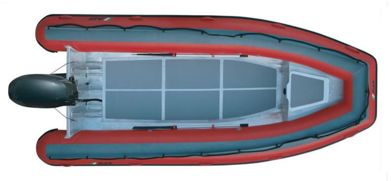
**Overal Length** : 16'/ 4.88m Number of Chambers : 5 Shaft Length : 20" / 50.8cm **Overal Beam** : 7'/ 2.14m **Person Capacity** : 10 RDC Design Category : C Inside Length : 12'8"/3.85m Weight : 480lb/218kg : 50hp/37.3kw Inside Beam : 3'6"/ 1.08m Recommended HP **Tube Diameter** : 21"/ 0.53m Maximum HP : 60hp / 44.8kw
