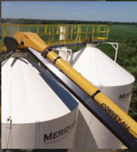
The 1600 Series uses a 16" belt inside a 10" tube, and is available in 35' to 100' lengths. They have a capacity of up to 6,000 bu/hr.
