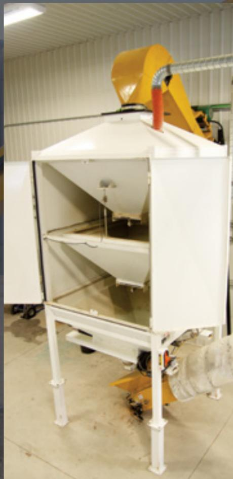
Our Surge Bin is designed to be temporarily or permanently set up. It has a 150 bu capacity and can be increased to 250 bu with side wall extensions. Adjustable legs allow clearance for your seed treater.
