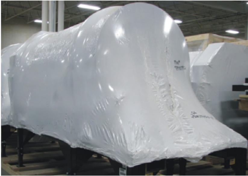
**Step 3:** Remove the protective covering from the Drum & Frame Assembly.
