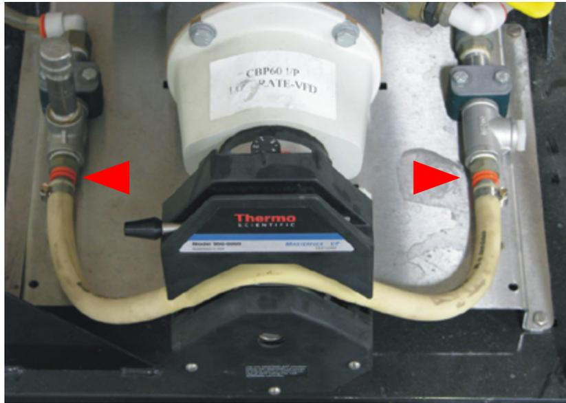
**Step 2:** Insert the Element press lock fitting into the Tank Elbow to the right of the Pump.
