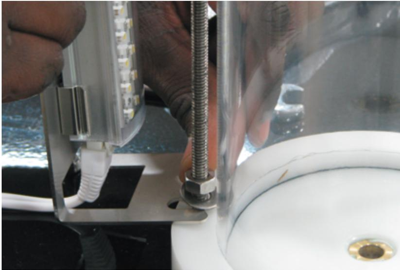
**Step 3:** Slide the Backlight Kit bracket under the lower nut and over the top stud.
