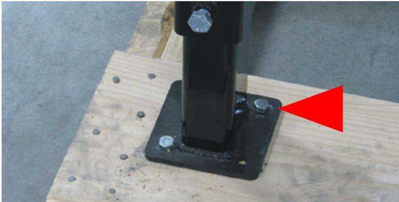
**Step 4:** Use a 3/4" socket head wrench to remove the 1/2" Drum Frame shipping bolts from the pallet.
