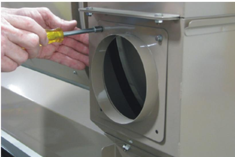
**Step 3:** Replace the Dust Collection Plate and securely fasten the four (4) 10-32 washers and bolts.
