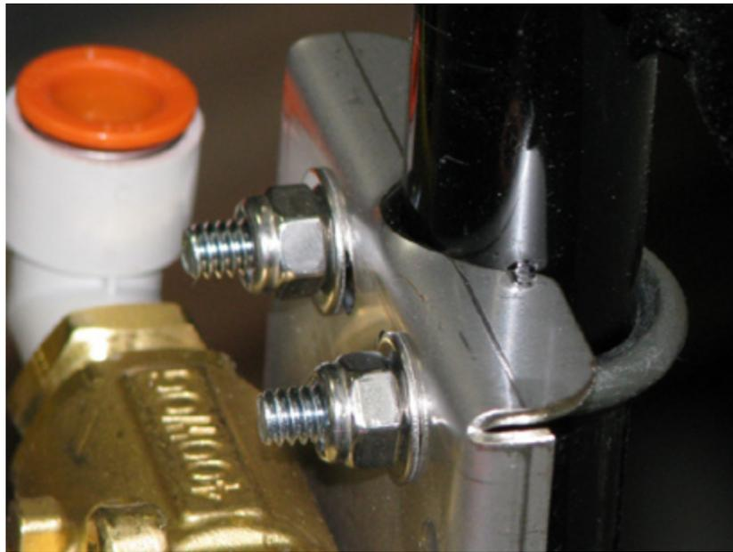
**Step 2:** Insert the U-bolt from behind the Tank Stand Frame and push through the Mount Plate.
