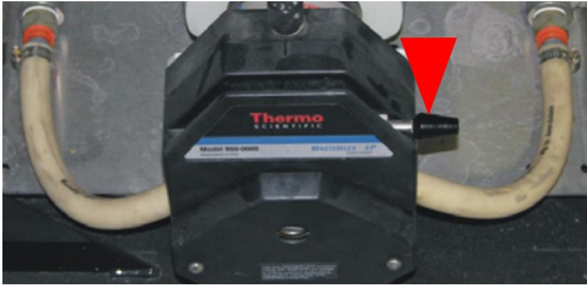
**Step 5:** Use the Pump Handle to close the Pump Head.
