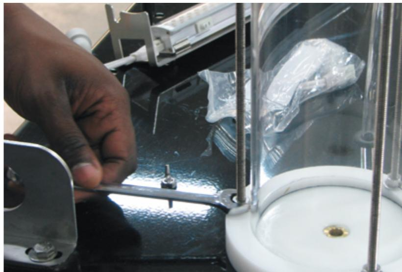
**Step 2:** Loosen the existing lower nut connected to the same stud as previous Step 1.
