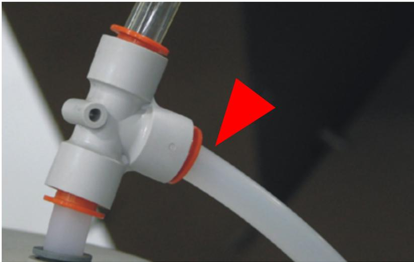
**Step 11:** Connect one end of the 1/2" Vent Tube to the 1/2" Union Tee.
