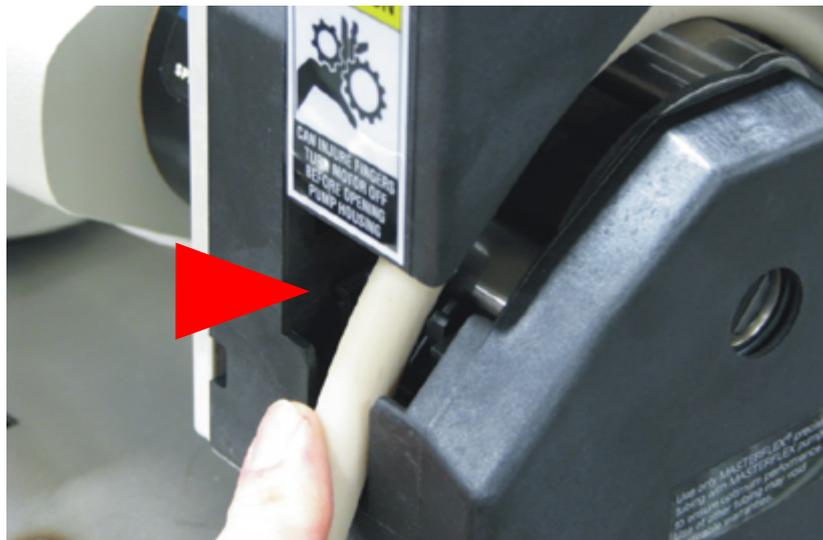
**Step 4:** Align the Pump Element on the Pump Head grooves to ensure a proper fit, as shown (may require two people).
