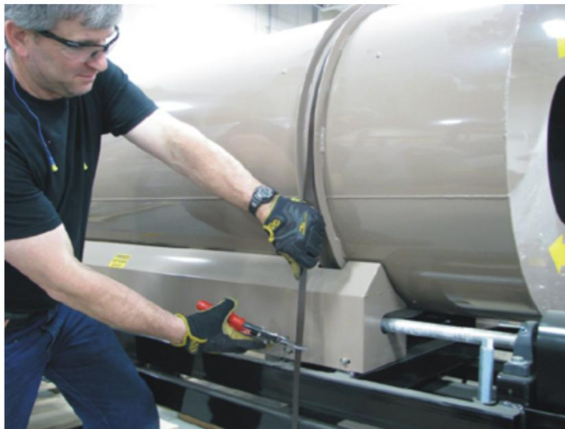
**Step 6:** Use tin snips to cut the metal banding that holds the Drum down onto the Drum Frame during shipping.
