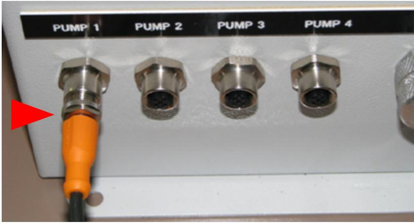
**Step 4:** Connect the other end of the signal cable to bottom of the 4-Pump Display Box.
