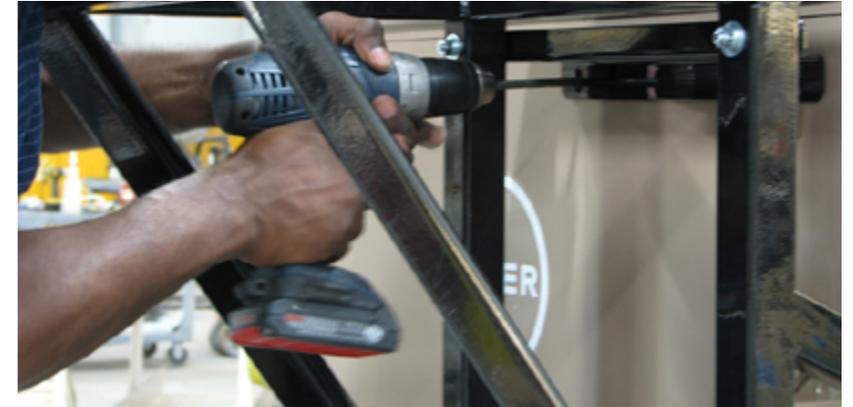
**Step 11:** Remove shipping bolts that hold the Powder Feeder Assembly onto the pallet.
