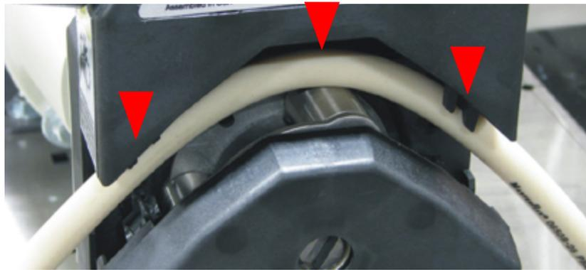
**Step 3:** Insert the factory supplied Pump Element onto the Pump Rollers.
