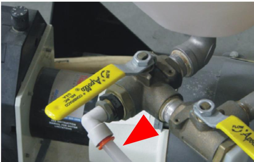
**Step 12:** Cut to fit and connect the other end of the Vent Tube to the 1/2" Press-lock Fitting on the pump, located underneath the Tank.
