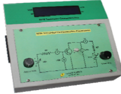
CE Amplifier Characteristics experiment setup
