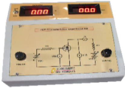
FET Characteristics experiment setup
