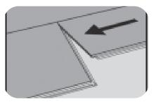
After installing the first piece of the secondrow, click the long joint of the plank Into the previous row and slide it into place
