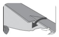
Lower the plank down flat, using a mallet to tap the small joint down into place (A tapping block may be required to lock plank into long edge)
