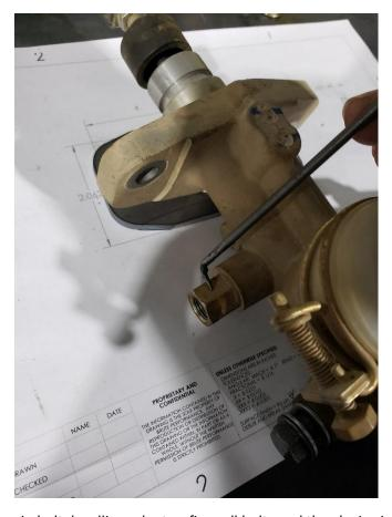
You will reuse the banjo bolt, hardline adapter, firewall bolts and the clevis pin on the brake petal
