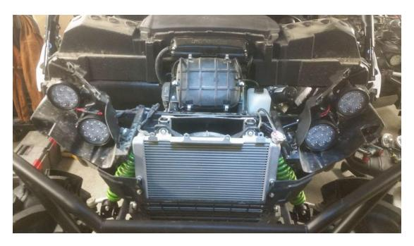
The new spacers have a flat side and an indent side. The flat side goes towards the light.
