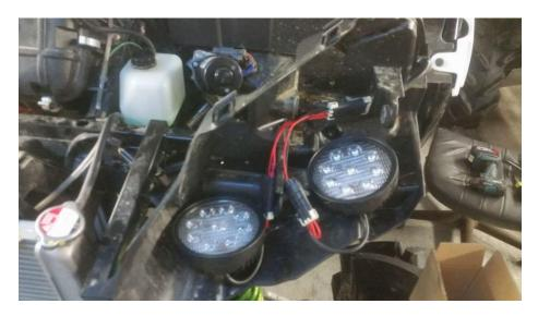
Connect the new lights to the new harness and use the provided spacers and bolts to assemble the bucket.
