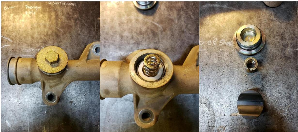
**Machine work to the cap should be performed on a lathe to ensure a centered straight hole**
