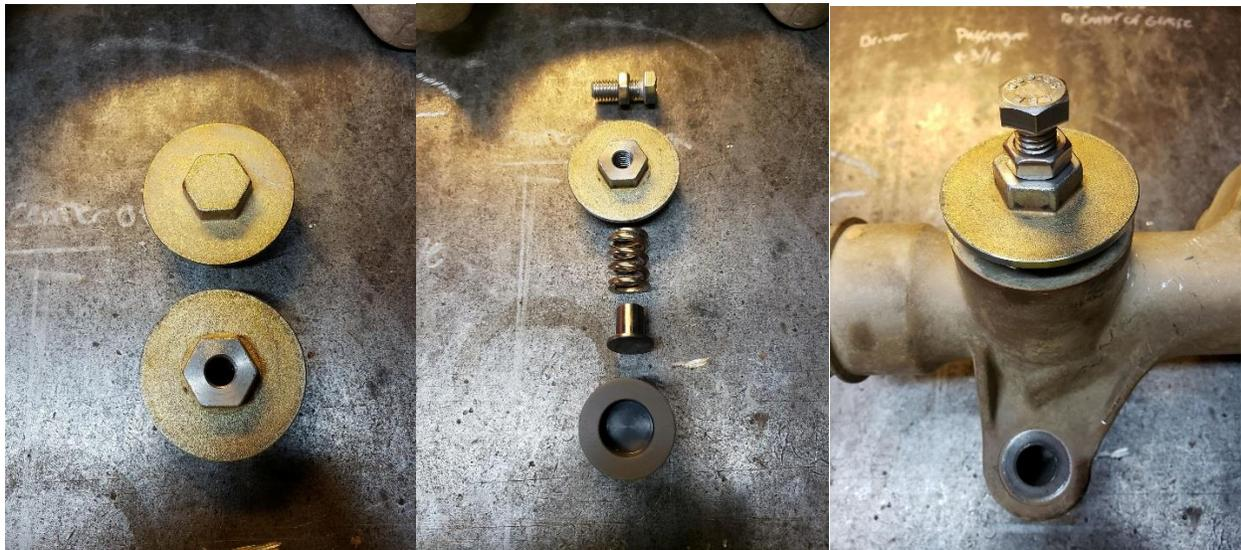
**Removal and installation of the bushing may require complete disassembly of the steering rack.**
