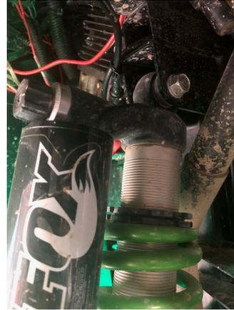
Once you've achieved this, begin installing the Bracket and Mounting bolt and spacer. The bolt simply passes through the brackets, A-arm and Spacer. Install the nut hand tight and then move on to the "Fat Washers" and the Lower shock mounting bolt. Once the washers and shock are installed, just hand tighten the mounting bolt and you can then begin the preload adjustment process. (IF you have decided to go this route..)
